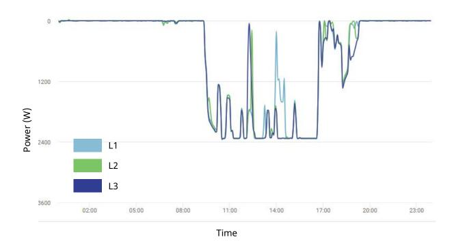
Further, in a scenario where the surplus PV energy exceeds the household energy demand but is not limited by a feed-in limitation, the secondary goal of the inverter is to restore symmetry at the <u>inverter</u> <u>output</u> as closely as possible. However, it's important to note that the aim is <u>not to keep up symmetry</u> <u>at the grid transfer point</u>. The following figure illustrates this scenario.
