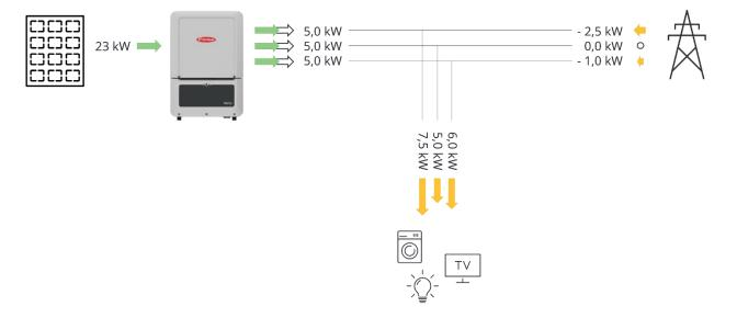
With the introduction of asymmetrical generation, it's now possible to precisely match the production to the demand on each phase while still ensuring zero physical feed-in.
