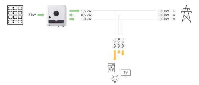
Example of Symo GEN24 10.0 Plus incl. battery & Ohmpilot with <u>a</u>symmetric generation and 2,33 kW feed-in limitation per phase: In night-hours, energy consumption from the grid is prevented efficiently and household loads are covered by the battery. In day-hours any feed-in to the grid is limited with 2,33 kW per phase (7 kW in total) and the inverter pushes its production towards this limit by compensating household loads with asymmetric generation.
