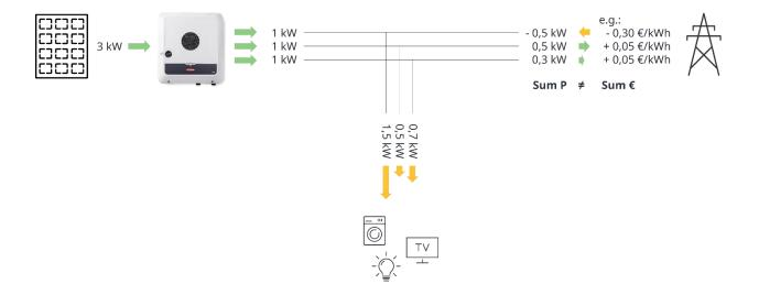
Example of Symo GEN24 10.0 Plus incl. Battery & Ohmpilot with <u>symmetric</u> generation and feed-in limitation of 7 kW: In night-hours, energy is exported to the grid on certain phases and consumed on other phases, while the sum of the energy flows remains zero. In day-hours, feed-in to the grid is limited with 7 kW in total, but exceeds 2,33 kW (33% of 7kW) on some phases as a result of household load asymmetry.
