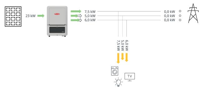
This innovative approach not only optimizes energy production but also ensures compliance with zerofeed-in regulations. By dynamically adjusting the power output on each phase, the asymmetrical generation feature maximizes energy utilization while maintaining grid compliance.
